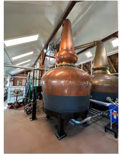
Above, top to bottom: Tenmile Distillery located on Sin Patch Road in Wassaic is surrounded by gardens, fields, and an apple orchard. Photo courtesy of Tenmile Distillery. Tenmile’s sculptural copper Forsyth stills were imported from Scotland and installed by Scottish technicians. Left: At the end of the Tenmile tour visitors congregate in the congenial bar for cocktails and sampling. Photos by Christine Bates.
